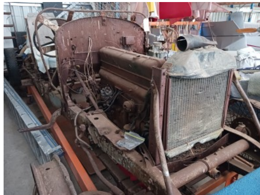
The remains of Squizzy Taylor's 1920's Buick, bought and modified into a glider launch winch.
